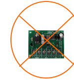
No charge controller unless 20 Watt panel or above
