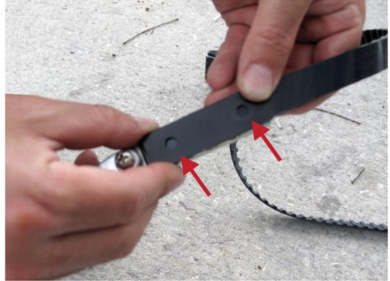
Attach the assembled belt bracket to the belt attachment bolt.
