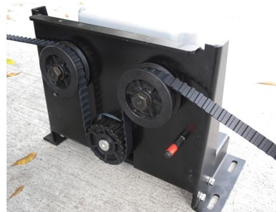
Make your final tightening adjustments on the belt. The belt should not have excessive sag in it (no more than 2 inch variance from furthest bracket to opener). To tighten the belt after mounting, move the nuts on the belt attachment bolt.
