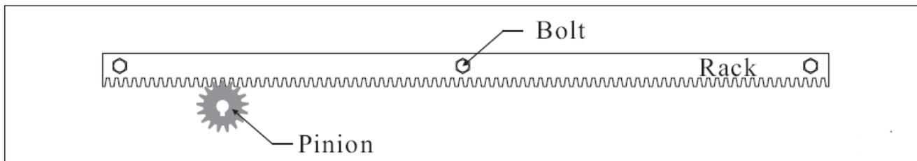
3. Move the gate manually, checking if the rack is resting on the pinion. Repeat at each hole.
