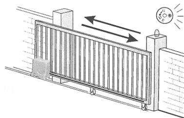
**Note: If your gate moves further open instead of closed: the motor side is incorrect.**
