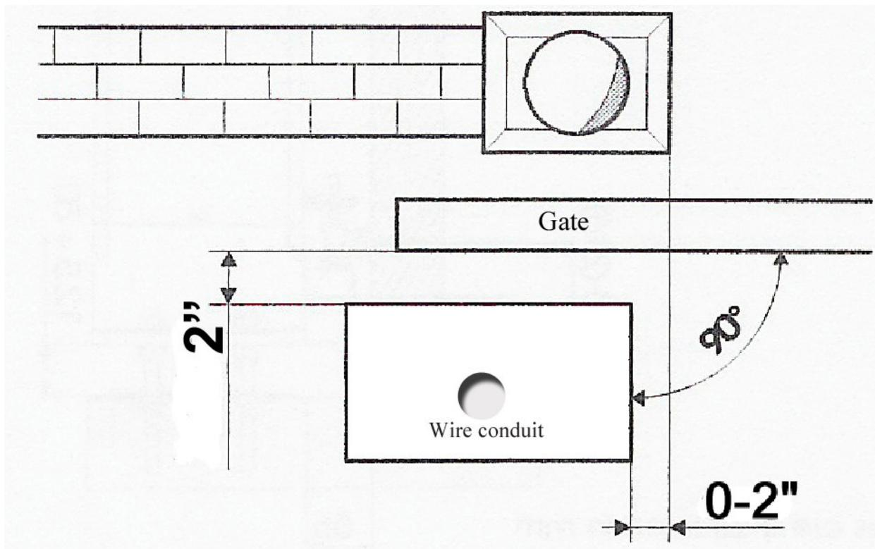
**Concrete Slab Tips:** Creating a wood rectangle with no top is a good way to form a slab. After the cement dries the wood can be knocked away. The slab must be secured to the ground below. Having rebar pass into the slab works well.
