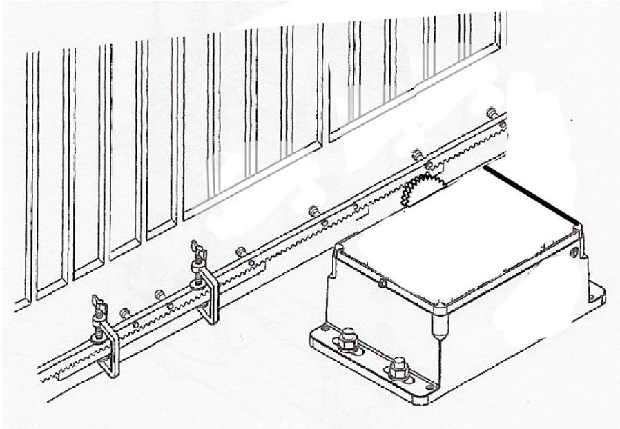
5. Move the gate manually and carry out the securing operations as far as the first element, proceeding until the gate is fully covered.
